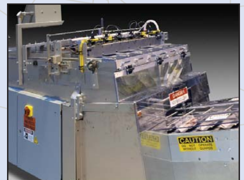
After slicing, the lane sorter distributes product into six lanes
